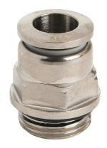
NITRA pneumatic push-to-connect fitting, straight, nickel-plated brass body, nickel-plated brass threads, thread sealant, (1) G3/8 male BSPP to (1) 3/8in push-to-connect. Package of 5.
