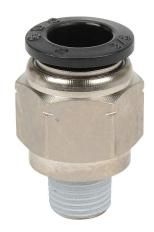
NITRA pneumatic push-to-connect fitting, straight, nickel-plated brass body, nickel-plated brass threads, thread sealant, (1) 1/8in male NPT to (1) 3/8in push-to-connect. Package of 5.
