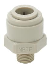
HydroMode potable water push-to-connect fitting, male, straight, acetal body, acetal threads, (1) 3/8in tube to (1) 1/8in male NPT connection(s), NSF/ANSI 61. Package of 5.
