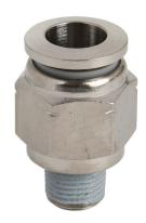
NITRA pneumatic push-to-connect fitting, male, straight, nickel-plated brass body, nickel-plated brass threads, thread sealant, 3/8in push-to-connect to 1/8in NPT. Package of 5.
