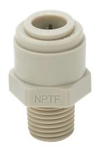
HydroMode potable water push-to-connect fitting, male, straight, acetal body, acetal threads, (1) 3/8in tube to (1) 1/4in male NPT connection(s), NSF/ANSI 61. Package of 5.
