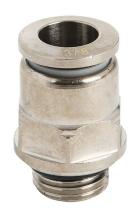
NITRA pneumatic push-to-connect fitting, straight, nickel-plated brass body, nickel-plated brass threads, thread sealant, (1) G1/4 male BSPP to (1) 3/8in push-to-connect. Package of 5.
