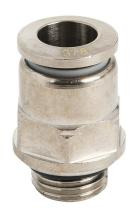
NITRA pneumatic push-to-connect fitting, male, straight, nickel-plated brass body, nickel-plated brass threads, thread sealant, 3/8in push-to-connect to G1/4 BSPP. Package of 5.
