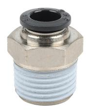
NITRA pneumatic push-to-connect fitting, straight, nickel-plated brass body, nickel-plated brass threads, thread sealant, (1) 1/2in male NPT to (1) 3/8in push-to-connect. Package of 5.
