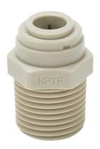
HydroMode potable water push-to-connect fitting, male, straight, acetal body, acetal threads, (1) 3/8in tube to (1) 1/2in male NPT connection(s), NSF/ANSI 61. Package of 5.
