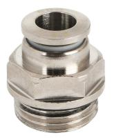
NITRA pneumatic push-to-connect fitting, straight, nickel-plated brass body, nickel-plated brass threads, thread sealant, (1) G1/2 male BSPP to (1) 3/8in push-to-connect. Package of 5.
