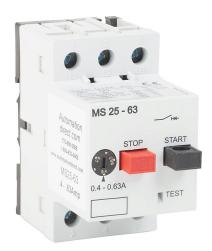
AutomationDirect MS25 series manual motor protector, pushbutton, 0.63A, thermal overload, 0.4-0.63A adjustable, 8A instantaneous trip rating, open, 45mm frame.
