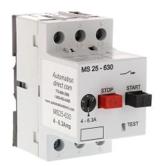
AutomationDirect MS25 series manual motor protector, pushbutton, 6.3A, thermal overload, 4.0-6.3A Adjustable, 75A instantaneous trip rating, open, 45mm frame.
