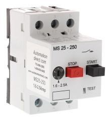
AutomationDirect MS25 series manual motor protector, pushbutton, 2.5A, thermal overload, 1.6-2.5A adjustable, 33A instantaneous trip rating, open, 45mm frame.
