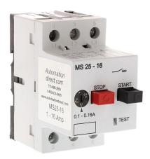
AutomationDirect MS25 series manual motor protector, pushbutton, 0.16A, thermal overload, 0.1-0.16A adjustable, 2A instantaneous trip rating, open, 45mm frame.
