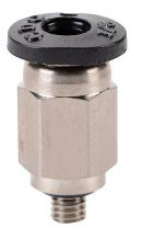
NITRA pneumatic push-to-connect fitting, straight, nickel-plated brass body, nickel-plated brass threads, thread sealant, (1) M3 x 0.5 male ISO to (1) 1/8in push-to-connect. Package of 5.
