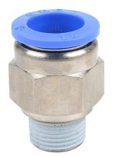
NITRA pneumatic push-to-connect fitting, straight, nickel-plated brass body, nickel-plated brass threads, thread sealant, (1) R3/8 male BSPT to (1) 16mm push-to-connect. Package of 5.
