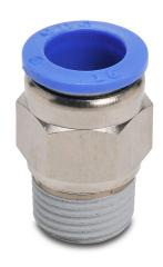
NITRA pneumatic push-to-connect fitting, straight, nickel-plated brass body, nickel-plated brass threads, thread sealant, (1) R1/2 male BSPT to (1) 16mm push-to-connect. Package of 5.
