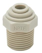
HydroMode potable water push-to-connect fitting, male, straight, acetal body, acetal threads, (1) 1/4in tube to (1) 3/8in male NPT connection(s), NSF/ANSI 61. Package of 5.
