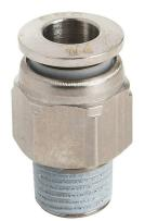
NITRA pneumatic push-to-connect fitting, straight, nickel-plated brass body, nickel-plated brass threads, thread sealant, (1) R1/8 male BSPT to (1) 1/4in push-to-connect. Package of 5.
