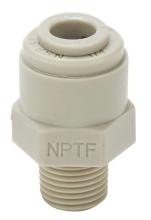
HydroMode potable water push-to-connect fitting, male, straight, acetal body, acetal threads, (1) 1/4in tube to (1) 1/8in male NPT connection(s), NSF/ANSI 61. Package of 5.
