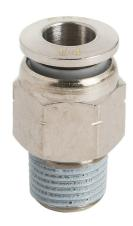
NITRA pneumatic push-to-connect fitting, straight, nickel-plated brass body, nickel-plated brass threads, thread sealant, (1) 1/8in male NPT to (1) 1/4in push-to-connect. Package of 5.
