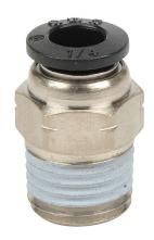
NITRA pneumatic push-to-connect fitting, straight, nickel-plated brass body, nickel-plated brass threads, thread sealant, (1) 1/4in male NPT to (1) 1/4in push-to-connect. Package of 5.
