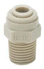
HydroMode potable water push-to-connect fitting, male, straight, acetal body, acetal threads, (1) 1/4in tube to (1) 1/4in male NPT connection(s), NSF/ANSI 61. Package of 5.
