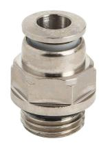
NITRA pneumatic push-to-connect fitting, straight, nickel-plated brass body, nickel-plated brass threads, thread sealant, (1) G1/4 male BSPP to (1) 1/4in push-to-connect. Package of 5.
