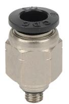
NITRA pneumatic push-to-connect fitting, straight, nickel-plated brass body, nickel-plated brass threads, thread sealant, (1) #10-32 male UNF to (1) 1/4in push-to-connect. Package of 5.
