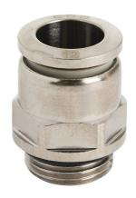
NITRA pneumatic push-to-connect fitting, straight, nickel-plated brass body, nickel-plated brass threads, thread sealant, (1) G3/8 male BSPP to (1) 12mm push-to-connect. Package of 5.
