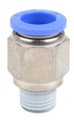
NITRA pneumatic push-to-connect fitting, straight, nickel-plated brass body, nickel-plated brass threads, thread sealant, (1) R1/4 male BSPT to (1) 12mm push-to-connect. Package of 5.
