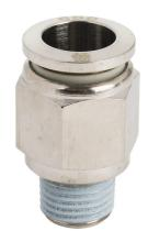
NITRA pneumatic push-to-connect fitting, straight, nickel-plated brass body, nickel-plated brass threads, thread sealant, (1) R1/4 male BSPT to (1) 12mm push-to-connect. Package of 5.
