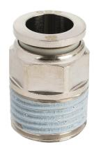
NITRA pneumatic push-to-connect fitting, straight, nickel-plated brass body, nickel-plated brass threads, thread sealant, (1) R1/2 male BSPT to (1) 12mm push-to-connect. Package of 5.
