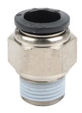
NITRA pneumatic push-to-connect fitting, straight, nickel-plated brass body, nickel-plated brass threads, thread sealant, (1) 3/8in male NPT to (1) 1/2in push-to-connect. Package of 5.
