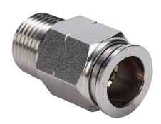
NITRA pneumatic push-to-connect fitting, straight, 316 stainless steel body, 316 stainless steel threads, (1) 3/8in male NPT to (1) 1/2in push-to-connect.
