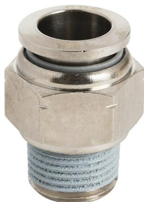
NITRA pneumatic push-to-connect fitting, straight, nickel-plated brass body, nickel-plated brass threads, thread sealant, (1) 3/8in male NPT to (1) 1/2in push-to-connect. Package of 5.
