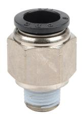
NITRA pneumatic push-to-connect fitting, straight, nickel-plated brass body, nickel-plated brass threads, thread sealant, (1) 1/4in male NPT to (1) 1/2in push-to-connect. Package of 5.
