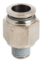
NITRA pneumatic push-to-connect fitting, straight, nickel-plated brass body, nickel-plated brass threads, thread sealant, (1) 1/4in male NPT to (1) 1/2in push-to-connect. Package of 5.
