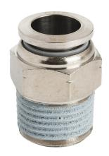
NITRA pneumatic push-to-connect fitting, straight, nickel-plated brass body, nickel-plated brass threads, thread sealant, (1) 1/2in male NPT to (1) 1/2in push-to-connect. Package of 5.
