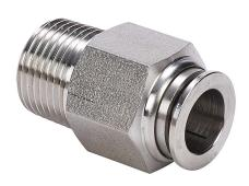
NITRA pneumatic push-to-connect fitting, straight, 316 stainless steel body, 316 stainless steel threads, (1) R3/8 male BSPT to (1) 10mm push-to-connect.
