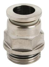
NITRA pneumatic push-to-connect fitting, straight, nickel-plated brass body, nickel-plated brass threads, thread sealant, (1) G3/8 male BSPP to (1) 10mm push-to-connect. Package of 5.
