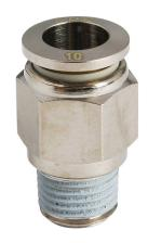
NITRA pneumatic push-to-connect fitting, straight, nickel-plated brass body, nickel-plated brass threads, thread sealant, (1) R1/4 male BSPT to (1) 10mm push-to-connect. Package of 5.
