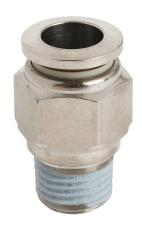
NITRA pneumatic push-to-connect fitting, straight, nickel-plated brass body, nickel-plated brass threads, thread sealant, (1) 1/4in male NPT to (1) 10mm push-to-connect. Package of 5.
