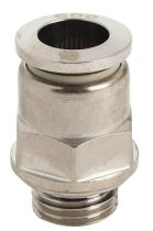
NITRA pneumatic push-to-connect fitting, straight, nickel-plated brass body, nickel-plated brass threads, thread sealant, (1) G1/4 male BSPP to (1) 10mm push-to-connect. Package of 5.
