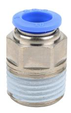
NITRA pneumatic push-to-connect fitting, straight, nickel-plated brass body, nickel-plated brass threads, thread sealant, (1) R1/2 male BSPT to (1) 10mm push-to-connect. Package of 5.
