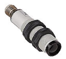
AutomationDirect photoelectric sensor, tubular, threaded, plastic, diffuse with background suppression, 100mm sensing distance, selectable light-on/dark-on, NPN/PNP, 80 Hz switching frequency, 4-pin M12 quick-disconnect.
