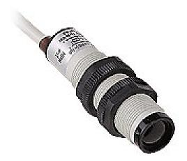
AutomationDirect photoelectric sensor, tubular, threaded, plastic, diffuse with background suppression, 100mm sensing distance, selectable light-on/dark-on, NPN/PNP, 80 Hz switching frequency, 6.5ft/2m cable length, pigtail.
