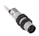
AutomationDirect photoelectric sensor, tubular, threaded, plastic, diffuse with background suppression, 100mm sensing distance, selectable light-on/dark-on, NPN/PNP, 80 Hz switching frequency, 6.5ft/2m cable length, pigtail.
