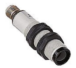
AutomationDirect photoelectric sensor, tubular, threaded, plastic, diffuse with background suppression, 50mm sensing distance, selectable light-on/dark-on, NPN/PNP, 80 Hz switching frequency, 4-pin M12 quick-disconnect.
