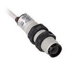
AutomationDirect photoelectric sensor, tubular, threaded, plastic, diffuse with background suppression, 50mm sensing distance, selectable light-on/dark-on, NPN/PNP, 80 Hz switching frequency, 6.5ft/2m cable length, pigtail.
