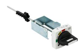
WEG Electric rotary handle, selector, black/gray, external front mount, 2-position, lockable in OFF only, defeatable, NEMA 4/4X, IP65. For use with MPW80 series manual motor protectors. 330mm shaft included.
