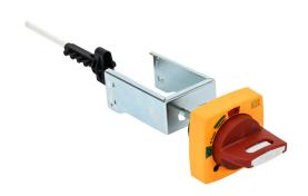
WEG Electric rotary handle, selector, red/yellow, external front mount, 2-position, lockable in OFF only, defeatable, NEMA 4/4X, IP65. For use with MPW80 series manual motor protectors. 330mm shaft included.
