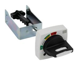
WEG Electric rotary handle, selector, black/gray, external front mount, 2-position, lockable in OFF only, defeatable, NEMA 4/4X, IP65. For use with MPW80 series manual motor protectors. 130mm shaft included.
