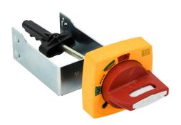
WEG Electric rotary handle, selector, red/yellow, external front mount, 2-position, lockable in OFF only, defeatable, NEMA 4/4X, IP65. For use with MPW80 series manual motor protectors. 130mm shaft included.
