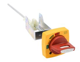
WEG Electric rotary handle, selector, red/yellow, external front mount, 2-position, lockable in OFF only, defeatable, NEMA 4/4X, IP65. For use with MPW40 series manual motor protectors. 330mm shaft included.
