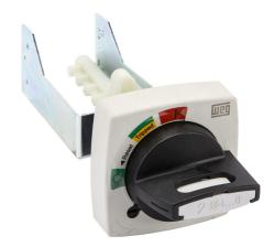
WEG Electric rotary handle, selector, black/gray, external front mount, 2-position, lockable in OFF only, defeatable, NEMA 4/4X, IP65. For use with MPW40 series manual motor protectors. 130mm shaft included.
